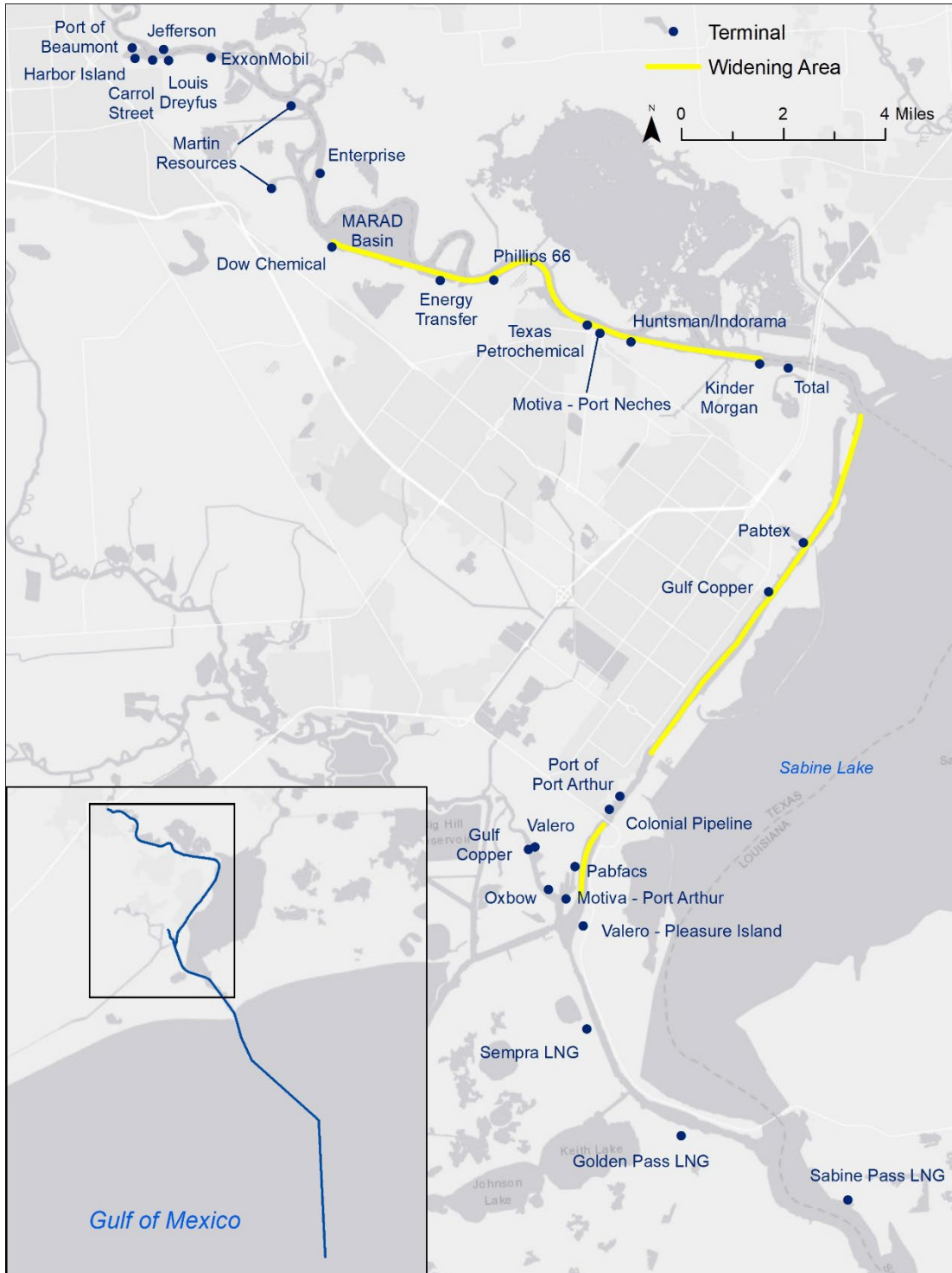
Figure E1 Widened Areas Under With-Widening Conditions
